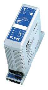
The MTL 9121-IS is a fieldbus repeater isolator which repeats the fieldbus signal from a safe area, Zone 2 fieldbus to an intrinsically safe fieldbus for connection to devices in Zone 1. The 9121-IS provides up to 120mA, typically powering up to 8 x 15mA field devices in Gas Group IIC.
